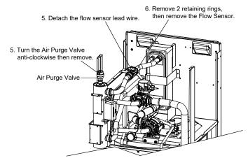
When reinstall Flow Switch, ensure the arrow on the flow switch is parallel with the pipe shaft and is facing in the direction of flow.
