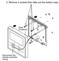
2. Disconnect the Remote Controller wiring.
