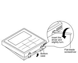
1. Remove the top case from the bottom case.
